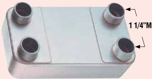
Art. S.010 - "AlfaMax" instantaneous heat exchanger, brazed stainless steel plate type, designed for high flow rates with parallel flow configuration. Connections: 1 1/4" M.
