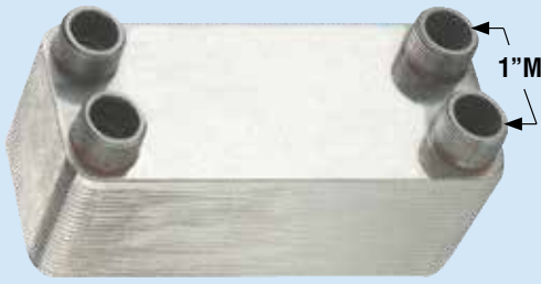
Art. S.009 - "AlfaMax" instantaneous heat exchanger, made of AISI 304 brazed stainless steel plates, designed for high flow rates with parallel flow configuration. Connections: 1" M.
