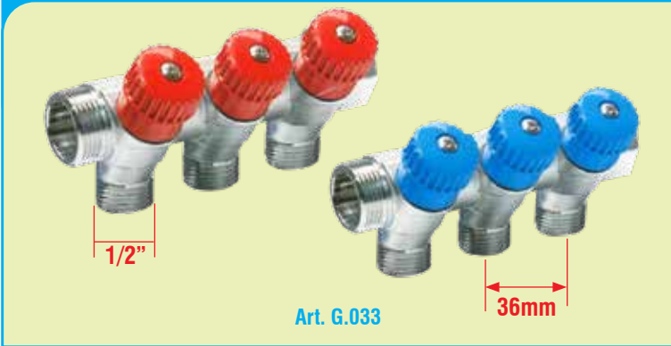
Art. G.033 - Modular, assembleable brass manifold with 1/2" M. branches. Center-to-center distance of the branches: 36 mm.
