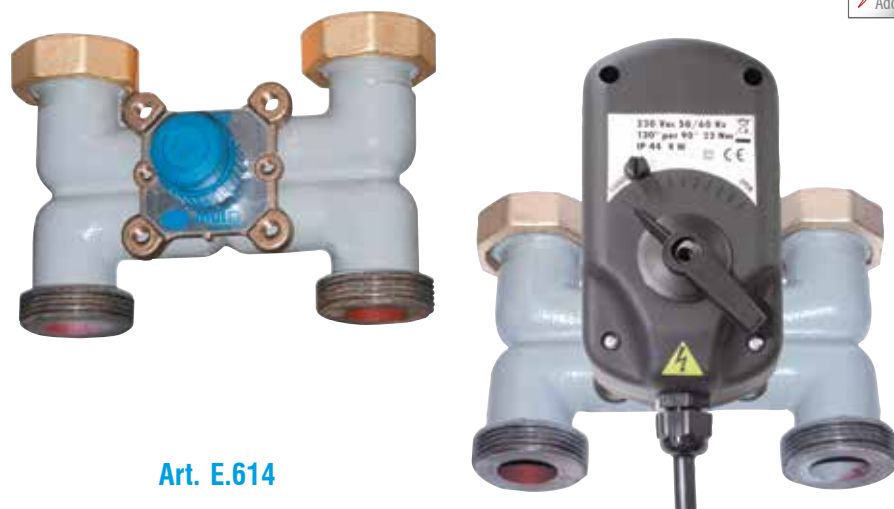
Art. E.614 – 4-way cast iron mixing valve cross-type with parallel connections 1 1/2" M. x 1 1/2" F. swivel.
