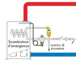
The valve should be installed only on horizontal pipe, with the obturator axis in vertical position. It is allowed the installation of the valve laying on the side (with the obturator axis in horizontal position) but never upside down.
