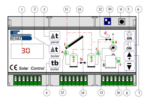
1) Display. Used to display all events that occur for programming by the user to read the temperatures detected by the probes.
